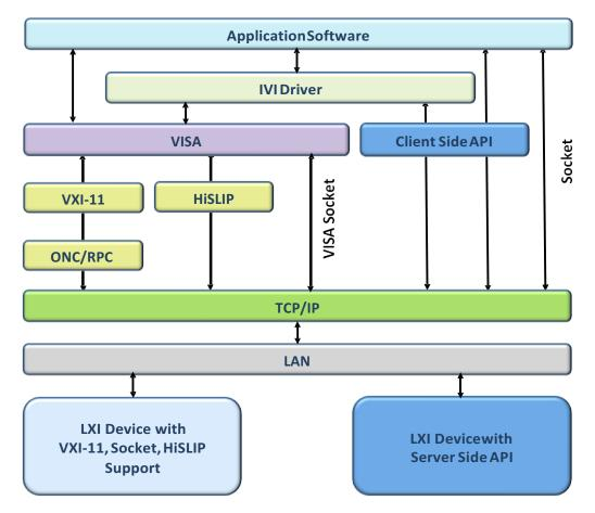
The LXI Reference Design focuses effort on the lower interaction between TCP-IP layer and the LXI Device's LAN interaction. It is a significant effort to implement the interactions between the layers of LAN protocol, provide LAN discovery, general communication, Web-page setup of proper LAN configuration, etc. The LXI Reference Design addresses these base and more advanced capabilities.
