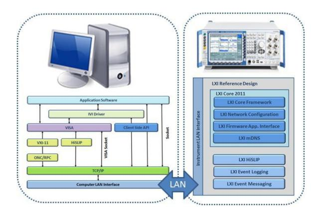
Basically the system design bases on the idea, that all LXI extended functions are placed in separate modules, which can be loaded independently during start-up. A small and simple LXI Core Framework handles this module concept. The communication between all modules is standardized and implemented in two separate classes (Provide Interface / Require Interface). The communication differs in asynchronous notification and synchronous commands/responses.
